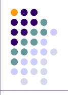
Factorization of a five-point matrix arising from Laplace PDE discretization.
