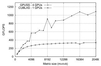
Performance near 1.1 TFlop (346 GFlops on 1 GPU using CUBLAS)
